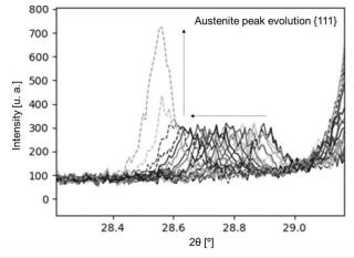
Figure 5.- Shift and growth of the main austenite peak {111} during heating
