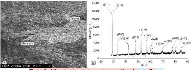
Figure 8.- Microstructure in tempering condition. A: SEM; B: XRD
