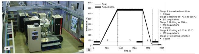
Figure 2.- A: Gleeble 3S50 equipment linked to the X-ray diffraction line; B: intercritical treatment cycle
