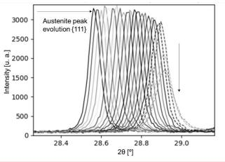
Figur 7.- Shift and decrease of the main austenite peak {111} during cooling
