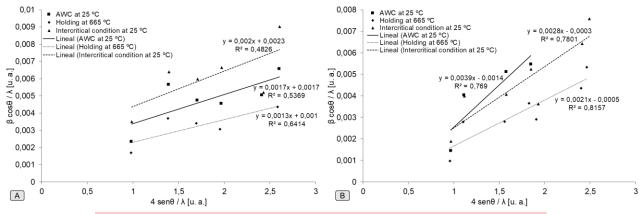
Figure 11.- Williamson-Hall method for A: martensite and B: austenite
