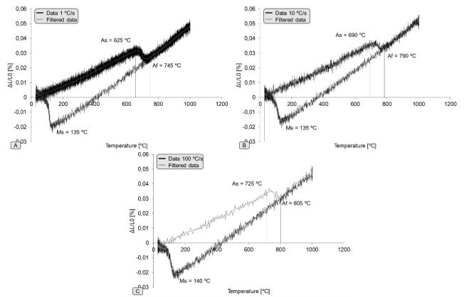
Figure 3.- Dilatometry curves for different heating rates. Filtered and real data
