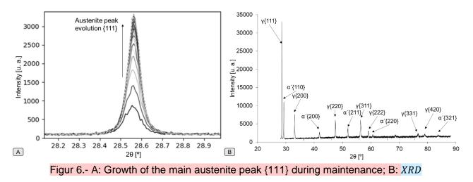
In this steel, this transformation behavior from martensite to austenite at constant temperature, was previously reported [25]. In dilatometry tests, the change in relative length during holding is greater for higher heating rates. These observations again imply the process being diffusional [25].
