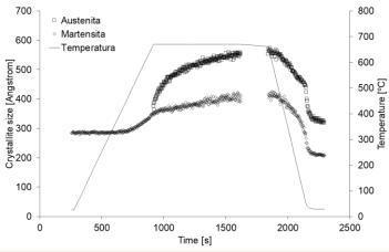
Figure 12.- Scherrer equation for martensite and austenite
