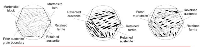
Figure 9.- Schemes of the microstructure in the different stages of heat treatment
